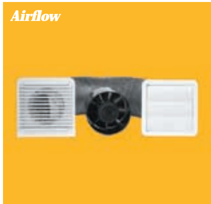
CE100D Kit Approximate Air Delivery 80m 3 /hour Power 15 Watts Duct Size 100mm
