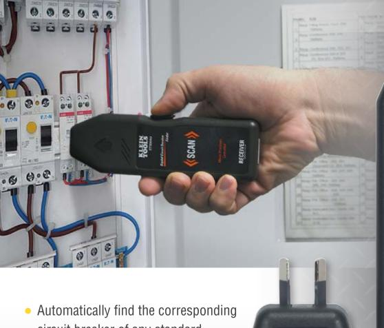
Automatically find the corresponding circuit breaker of any standard
