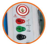
Line, V, Guard and Earth Interfaces
