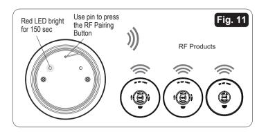
$\bullet$  To exit RF pairing mode, press the RF pairing button once. The red LED will turn off.
