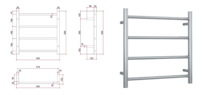
Note: All dimensions are in millimeters (mm)
