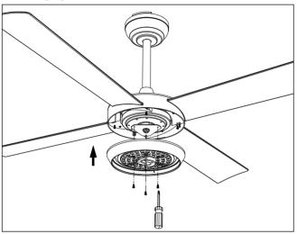
Install the LED light plate onto the steel bracket as illustrated with the 3 supplied screws.
