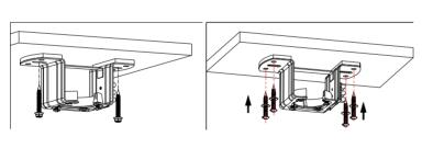
Secure the hanger bracket to ceiling beam or a suitable piece of timber inserted between the ceiling beams using the two long screws, or the four shorter screws supplied with the package.
