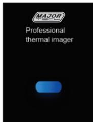
**Note:** After powering on, allow the MTi13 Thermal Imager a brief warm-up period for accurate temperature readings and optimal image quality. First, the visible image will appear, followed by a brief calibration of the thermal sensor. Once calibrated, the thermal image will display on the screen.
