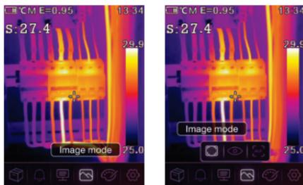
The Thermal Imager offers five display image modes: IR, Visible, Picture-in-Picture, AUF Mode, and Zoom Mode.
